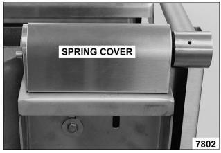
Place a 1 5/8" wrench on the lid spring lock nut and apply a downward force until locking pin can be removed. Continue to hold lock nut in place.
